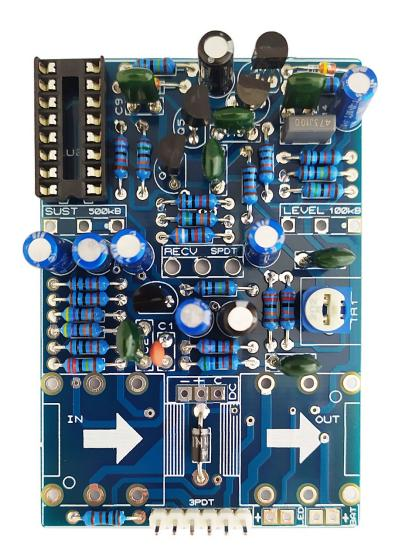
Solder the capacitors, transistors and the 2k trimmer. If you have troubles reading the values, check out our <u>"Reading Part Values"</u> tutorial. Pay attention to the orientation, as well as to the polarity for electrolytic capacitors.
