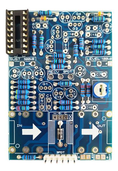
First of all place the IC socket (without the IC). Pay attention to the orientation! The small notch in the socket should be oriented as indicated in the PCB.
